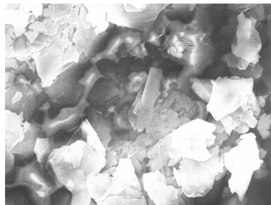
Fig. 6: SEM image of Graphite powder
